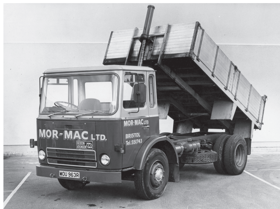
Commercial Motor's tester achieved 11.7mpg overall and a 10.6-tonne payload with a 200 in May 1977.
