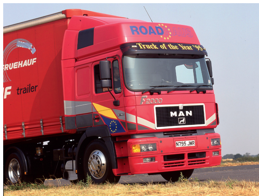
F2000 designations ended in "3". This is the 19.463 with the new 12.8-litre 460hp Euro-2 engine.
