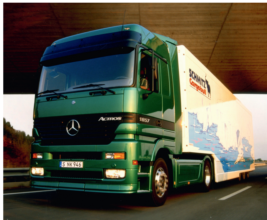
The 1857 was the flagship Actros – the V8 engine developed 571hp with 2,700Nm torque and there was 1.9m of standing room in the MegaSpace cab.
