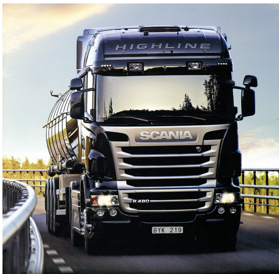
The Scania R 480, with 2,500Nm torque, revised Opticruise gearbox and 2.59:1 axle was a strong proposition for 44-tonne work.
