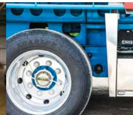
PSI inflation management and BroLube help keep the wolf from the door between formal tyre and maintenance visits.
