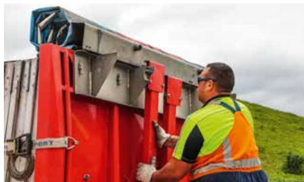
Adrian places the trailer posts and the cover rack hinges back down on top. Note the flip-latches that allow the whole thing to come off.
