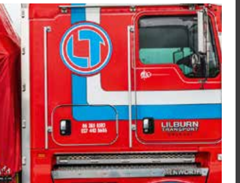
Blanked-out vent so as not to ruin the company logo, and a stainless light flash.
