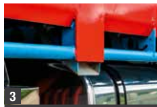
1) Rub pads on the sides prevent unsightly wear when stacked. 2) Springlocks prevent pin loss. 3) Angled post slots flick debris away from the shiny bits.
