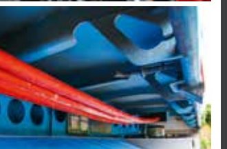
The unit is festooned with tie-down and lashing points. Full-length rope rails, vertical rope rails and chain hooks galore.
