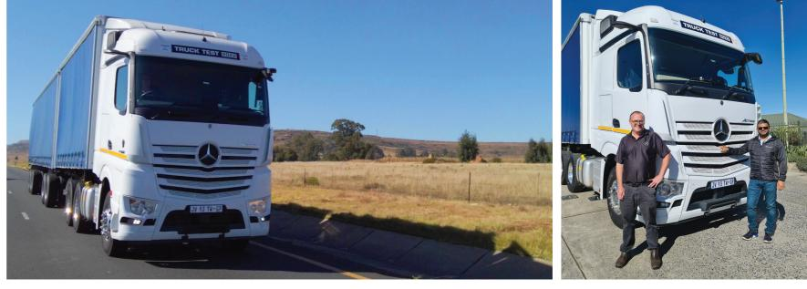
Predictive Powertrain Control (PPC). This highly innovative feature pre-emptively accelerates and decelerates the truck for best fuel economy when running in cruise control, based on the vehicle's instantaneous position using 3D map data.
