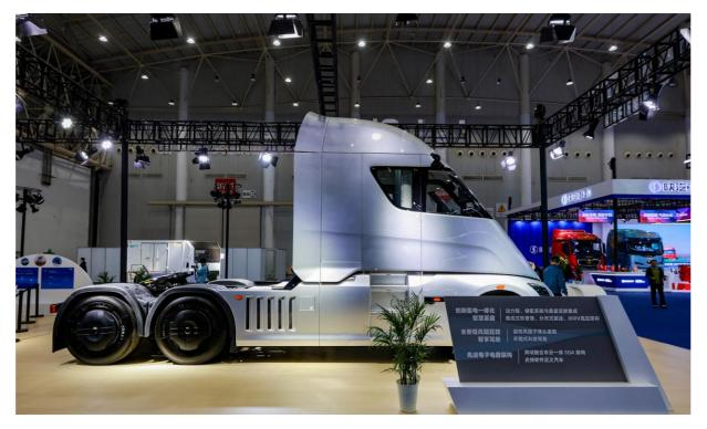
According to Sun Ying, under high-speed driving conditions with a full load of 49 tons, the hydrogen consumption of Hybot H49 can be as low as 7.1 kg/100 km, meeting the application scenarios of high-speed mainline logistics with a transport distance of 500-1,000 km.
